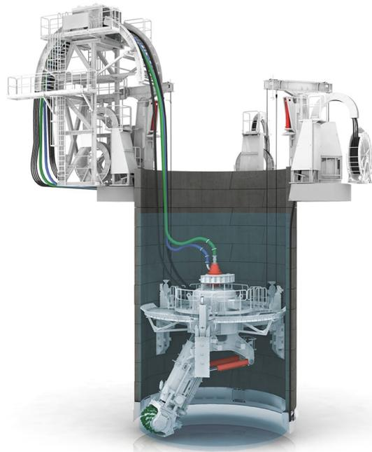
Fig. 7. Shaft boring machine [15]
