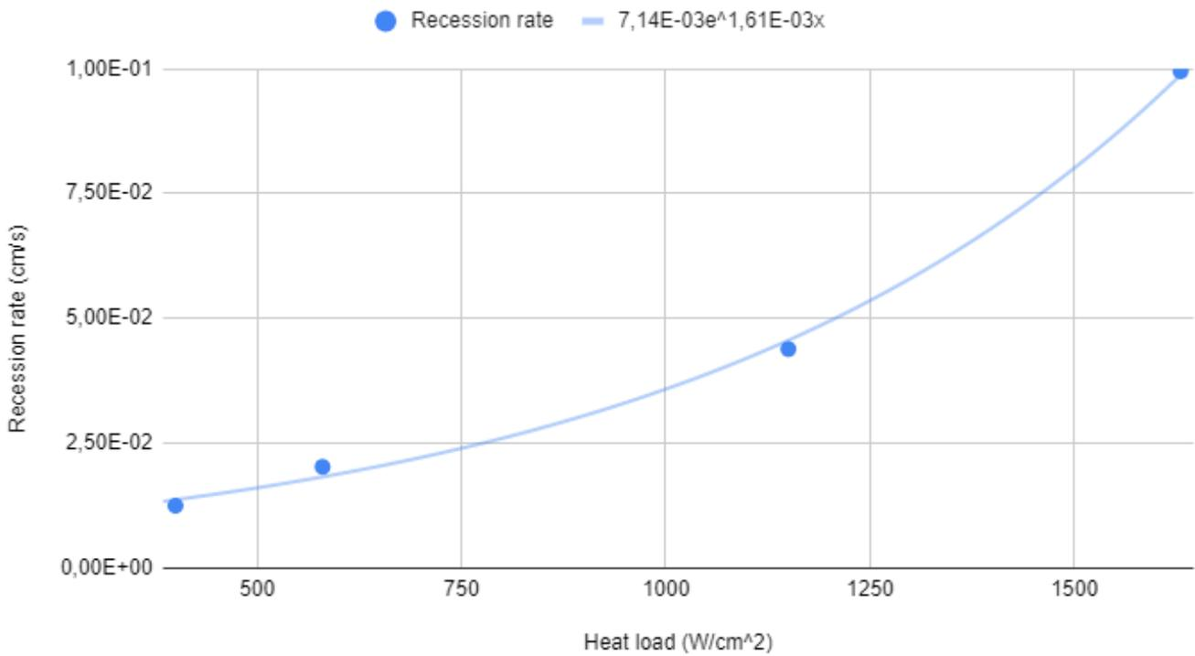
Figure 21: Ablation rate of low density ablative material
