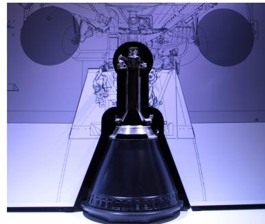
Fig. 2. Vinci rocket engine
