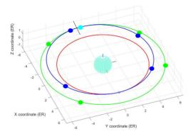
Figure 3: Hohmann Transfer between satellite 1 and satellite 2 both at GEO, but with an angle difference of  $9^{\circ}$ .
