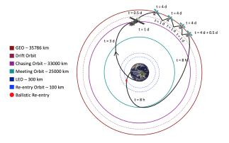
Figure 5: On-orbit operations with LEV, LSM, and SM.
