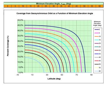
Figure 1: Evolution of Earth coverage with latitude and elevation angle, at GEO.
