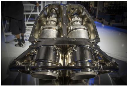
Fig. 7. SuperDraco engines. [3]
