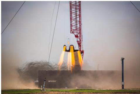
Fig. 8. Launch abort test for the Crew Dragon Capsule with the 4 pairs of SuperDraco engines. [3]
