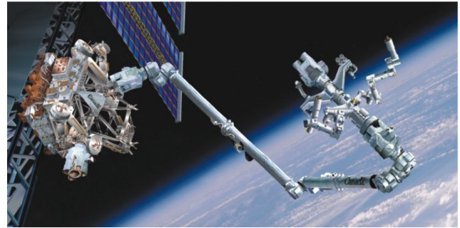
Fig. 9. The Mobile Servicing System, with from left to right: MBS, Canadarm 2, SPDM [16]
