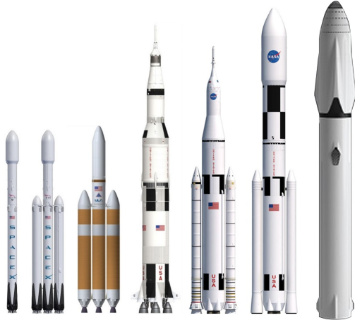
Fig. 2. Size Comparison of existing or planned super heavy launchers. From left to right: Falcon 9, Falcon Heavy, Delta IV Heavy, Saturn V, SLS Block 1, SLS Block 2, ITS
