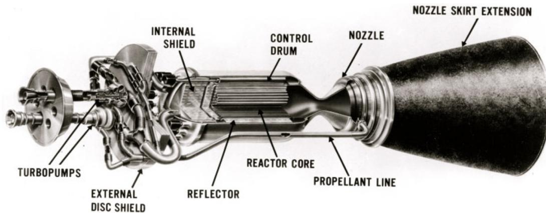
Figure 2. Schematic of NERVA-derived "Expander Cycle" NTR Engine [12]
