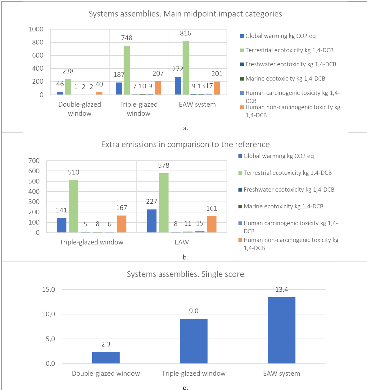
Figure 47 Systems assemblies comparison. a. Main midpoint impact categories for the three systems b. Extra midpoint emissions of System 2 and 3 due to a more complex system in relation to the reference. c. Single-score for the three systems
