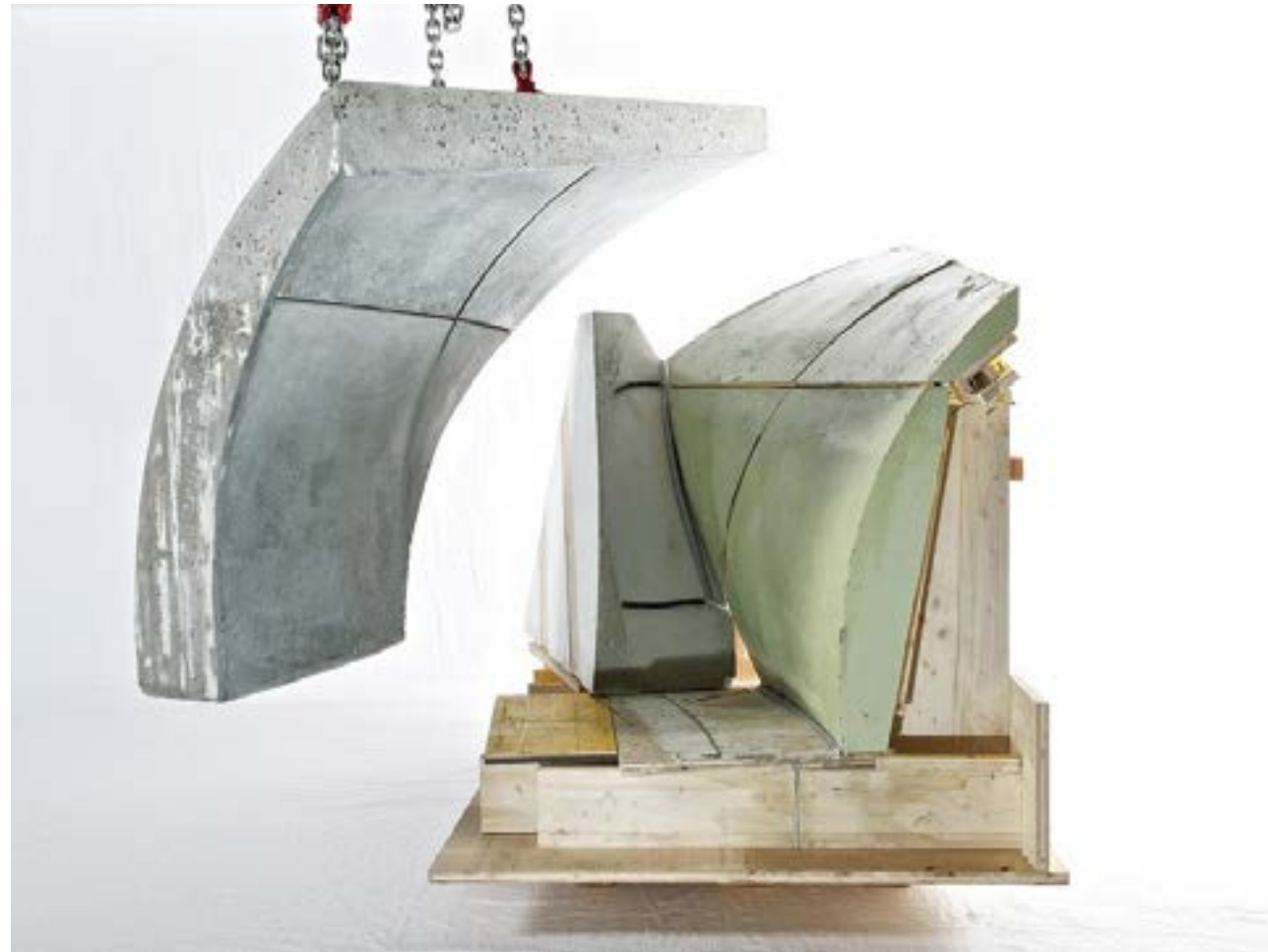
FIGURE 1.19 TailorCrete project, a zero-waste wax formwork for concrete (Source: ROK Rippmann Oesterle Knauss GmbH).
