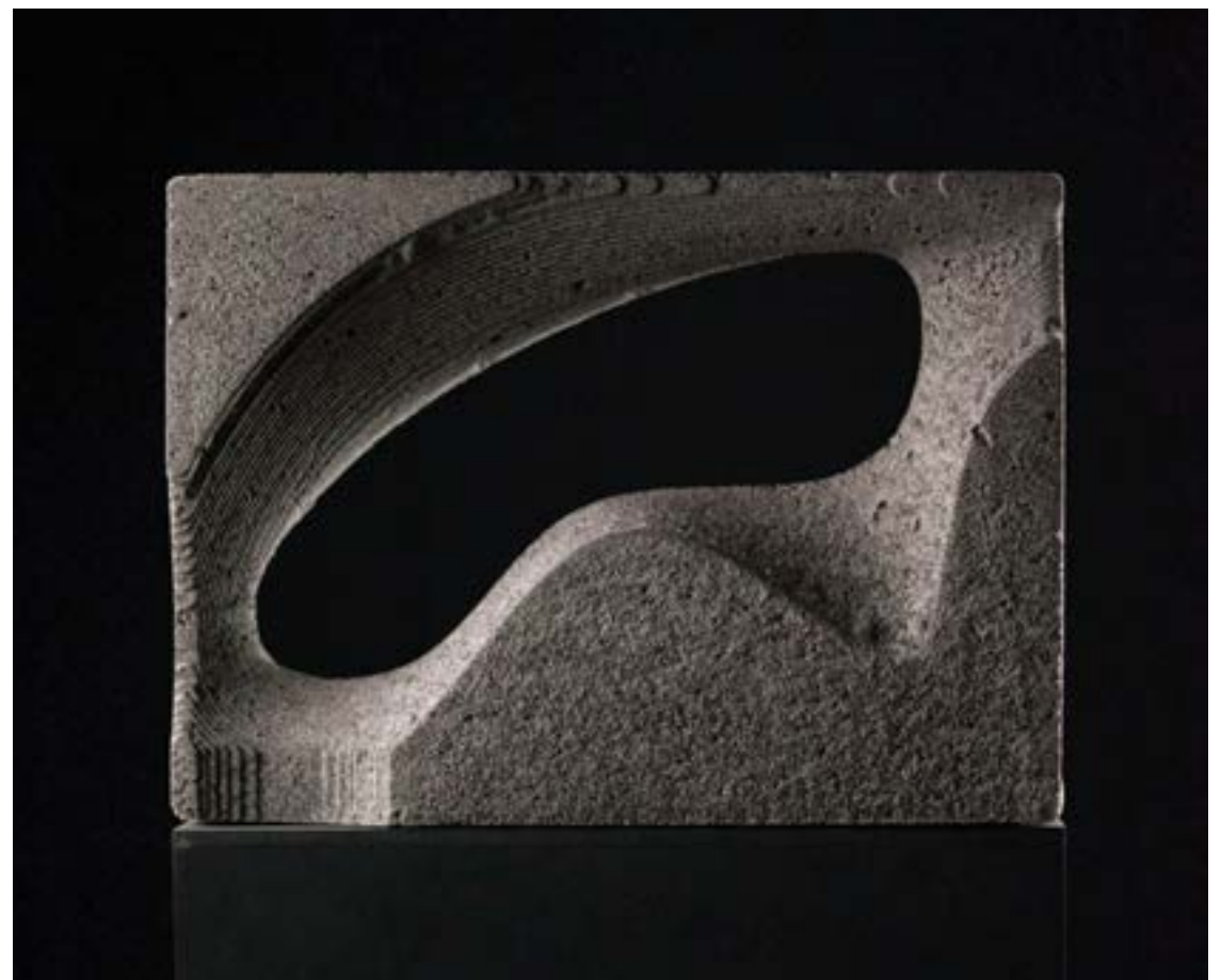
FIGURE 2.40 The prototype 180805-DP-APE1 made using a two-party ice mould assembly (Source: author).
