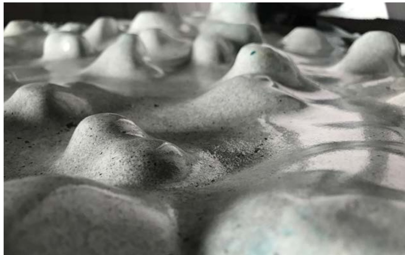
FIGURE 2.28 Ice mould for the concrete panel 170721-ME-MUR1 produced via thermal melting (see Film 2) (Source: author).
