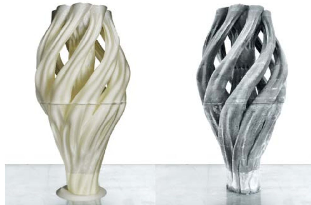
FIGURE 1.18 A concrete prototype cast in water-soluble 3D-printed PVA formwork (Source: Digital Building Technologies, ETHZ. Photo: Matthias Leschok).
