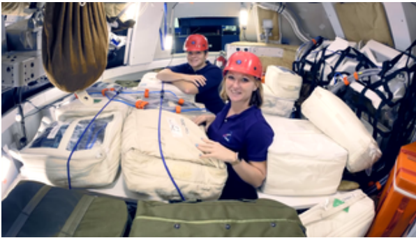
Fig. 4. Demonstration of the radiation protection plan in an Orion spacecraft mock-up. During an SPE, the crew will use stowage bags on board to create a denser shield against radiation.
