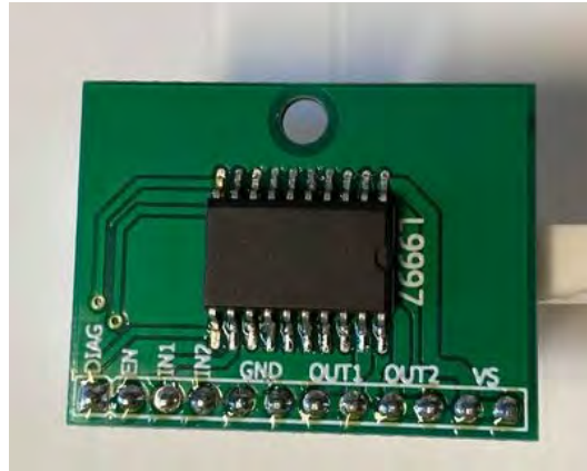
Figure 3.8. The H-bridge mounted on the front of the carriage.
