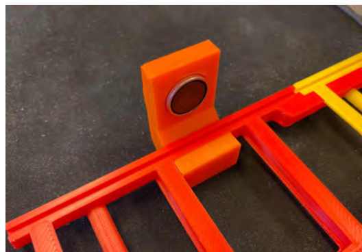
Figure 3.4. One of the magnets attached to the railway.
