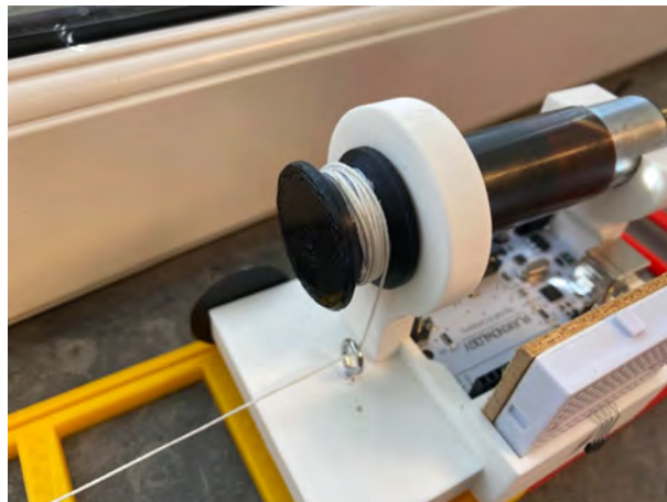
Figure 2.1. The winch used in this project
