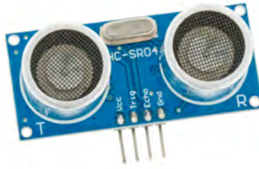
Figure 3.4. Ultra sonic sensor HC-SR04, [17]
