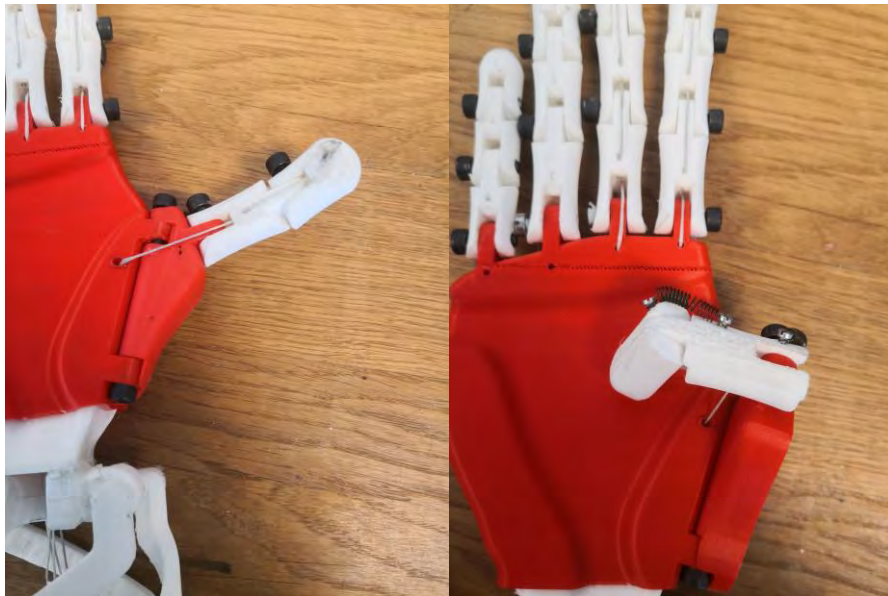
Figure 3.4: Thumb in its open and closed position (taken by authors)
