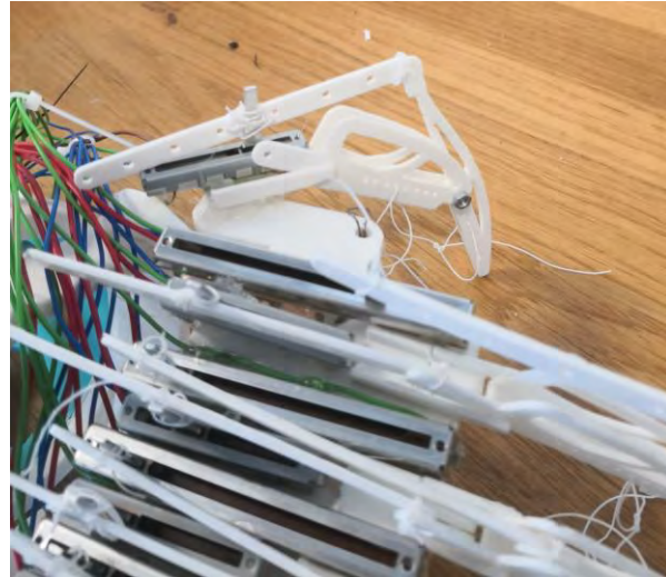
Figure 3.9: The potentiometers and back of hand (taken by authors)
