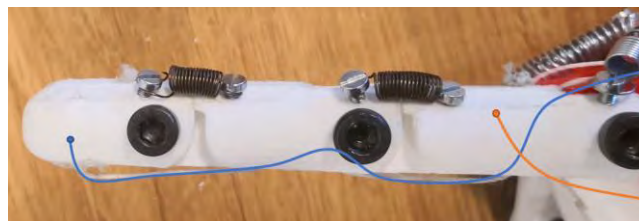
Figure 4.2: The springs and wires running through the finger (taken by authors)
