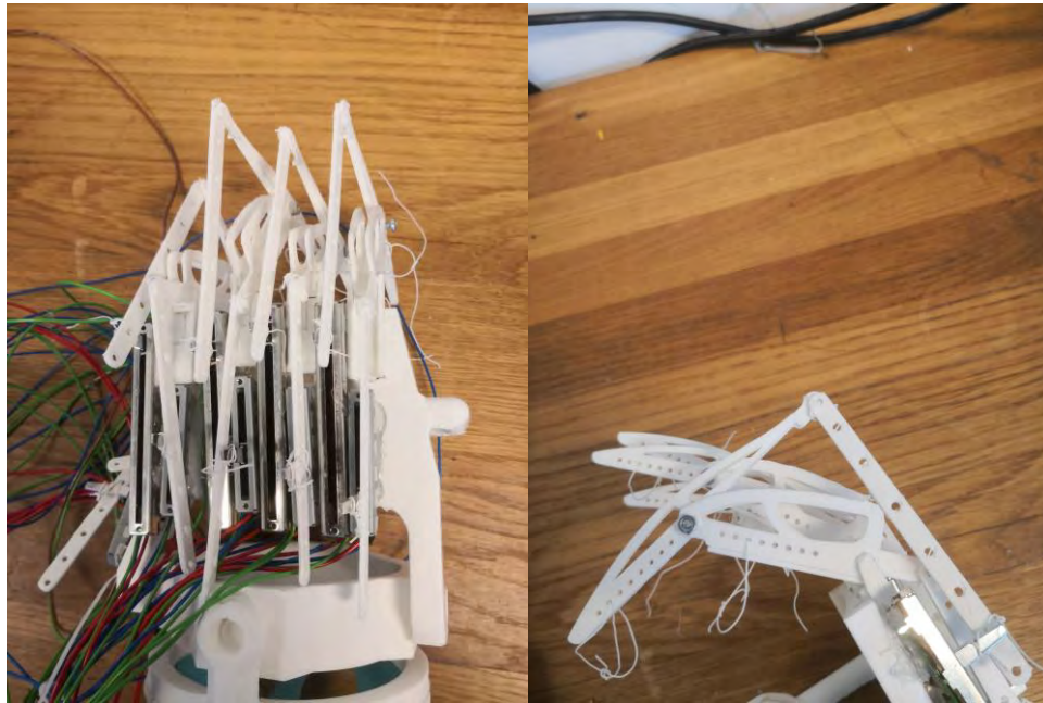
Figure 4.4: The finger assemblies (taken by authors)
