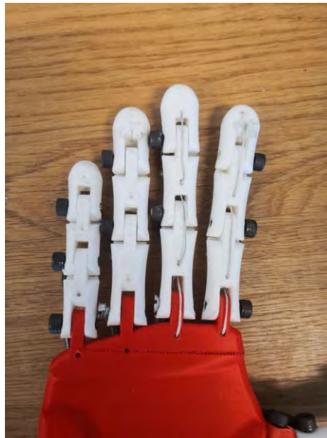
Figure 3.2: Hand and finger construction (taken by authors)
