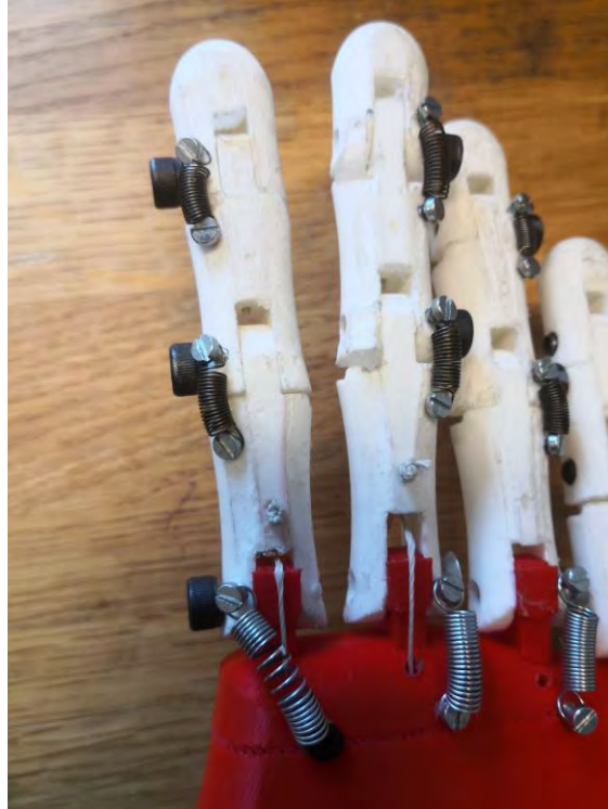
Figure 4.3: Springs at the back of the fingers (taken by authors)
