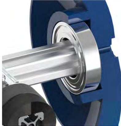
**Figure 3.3.** A CAD rendering of the bearings inside the Bowling ball. Created in Keyshot.
