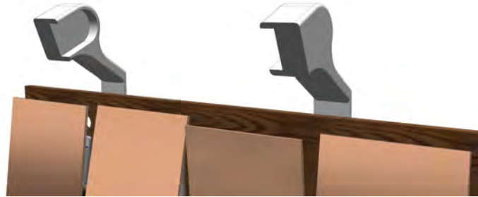
Figure 3.7. The two holders for the lamp fastened in the carrier (made with Solid Edge) [19].
