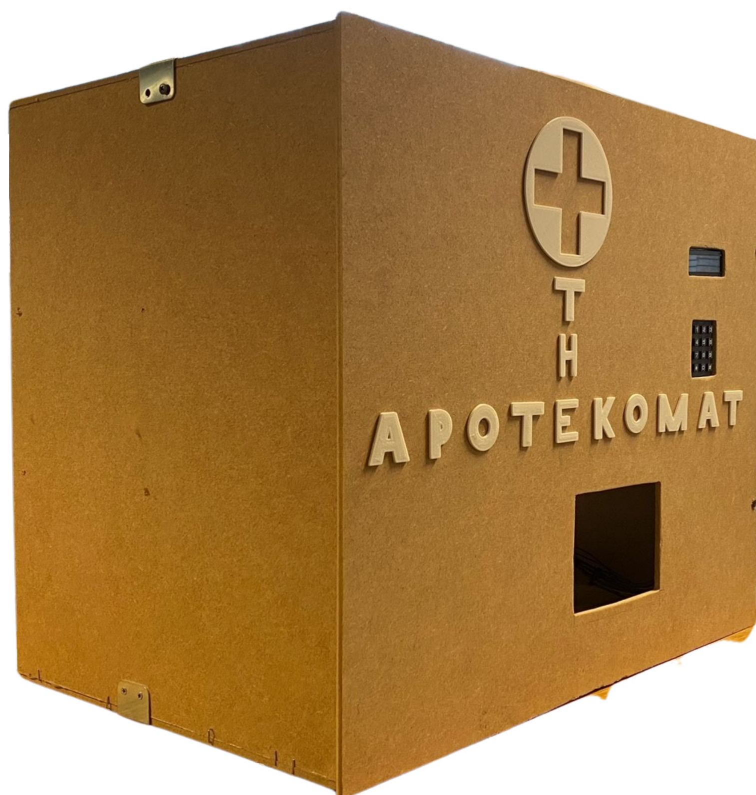
An overall picture of The Apotekomat's construction, the prototype delivers the medicine to the user after checking the user's data and password.
