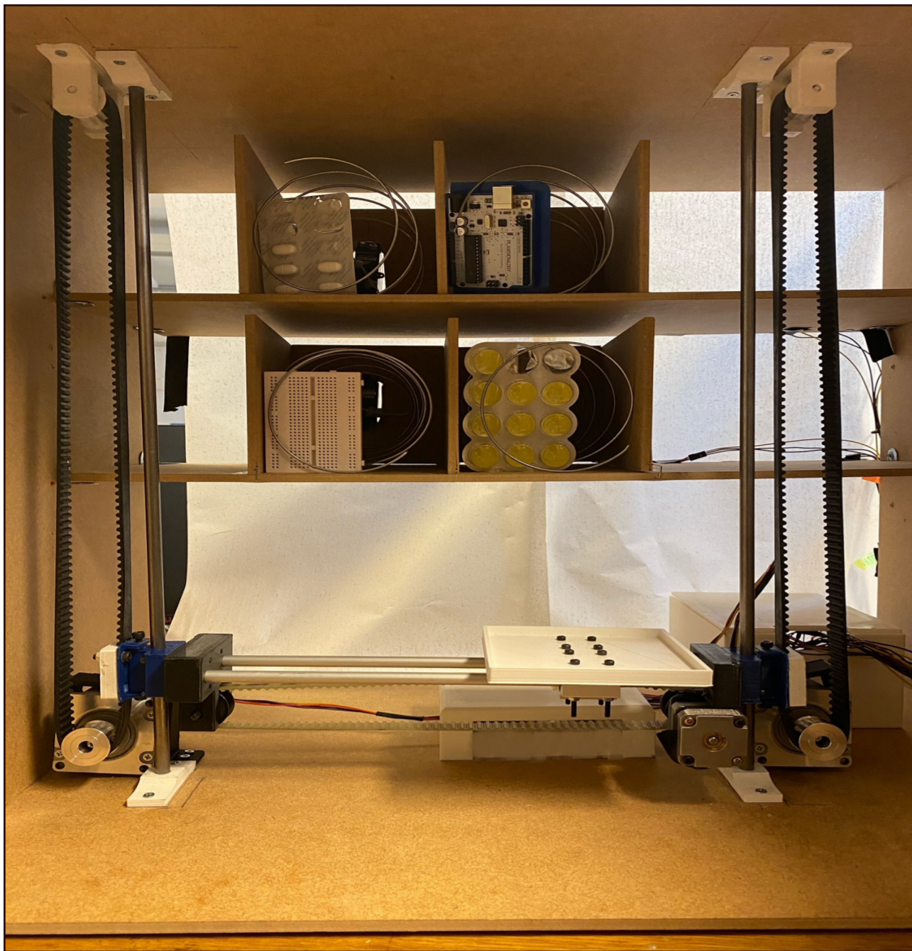
The internal construction of The Apotekomat.
