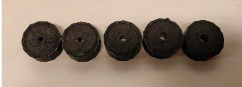
Figure 4.3: The nozzles that were used (4mm to 8 mm diameter from left to right). Picture taken by the authors
