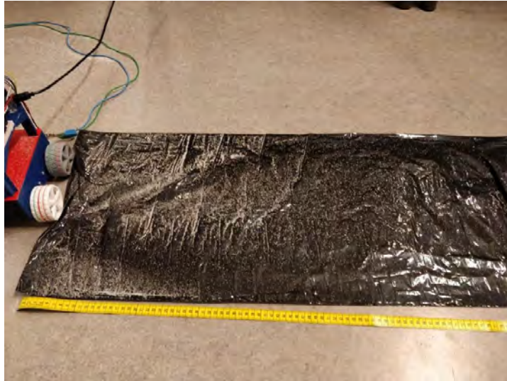
Figure 4.4: Testing of spread of the particles as a function of the rotational velocity of the DC motors. Picture taken by the authors
