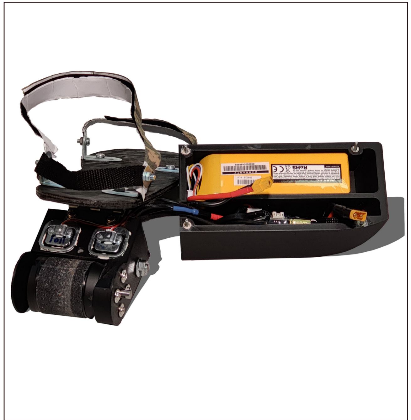
Internal view of electronics, load cells and electric motor.
