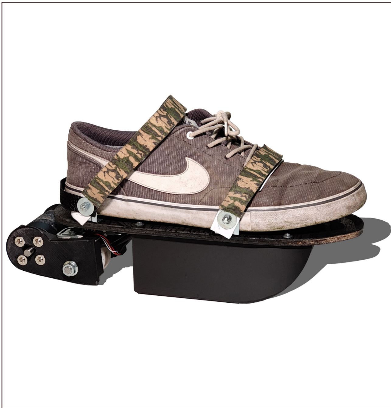
Final prototype. The user shifts weight onto the right foot to accelerate.
