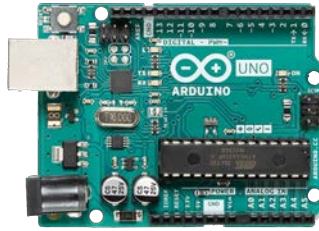
Figure 2.3. Picture of an Arduino Uno [8].
