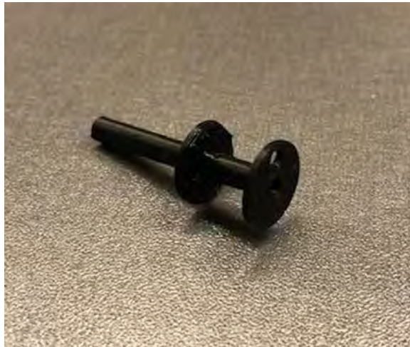
Figure 3.2. Spool to gather excessive fishing line, picture taken by authors.
