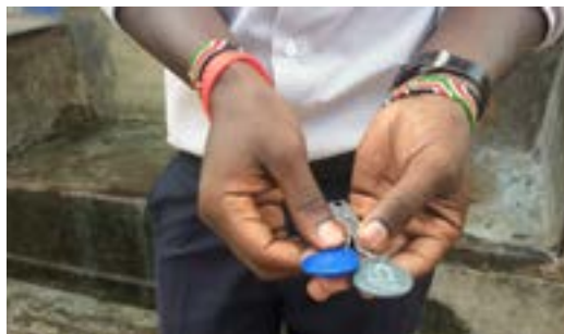
The electronic tokens used for payment on prepaid water meters in Nairobi. Photo: David Nilsson.
