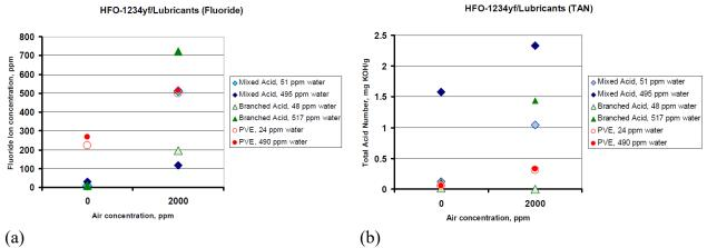
Figure 2 – Fluoride Ion Concentrations (a) and Total Acid Numbers (b) of Sealed Tubes Containing HFO-1234yf and Lubricants.
