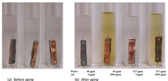
Figure 1 - Figure Photographs of Sealed Tubes Containing HFO-1234yf/ISO 32 Branched Acid Before (a) and After (b) Aging
