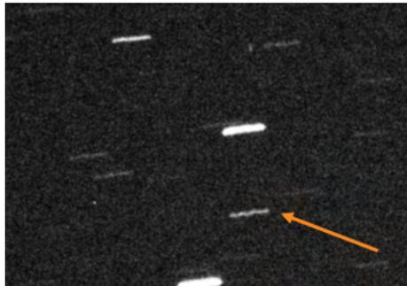
**Figure 2.5:** Example of mount vibrations disturbance in a satellite tracking image [24]. Mount vibrations cause the star tracklet to look zigzagged.
