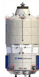
Fig. 11: ATV Propulsion system
