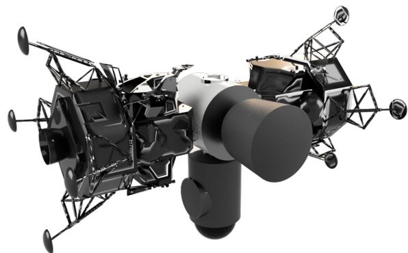
Fig. 7. CAD model of the node. On each side is a Mars descent vehicle (a model of the Apollo lunar lander is used as a placeholder). In the front is the earth descent capsule, and on the bottom is the EVA hatch and observation window.
