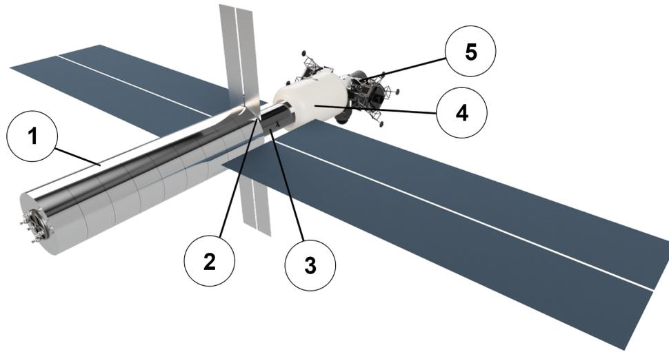
Fig. 9. CAD mock-up of the transfer vehicle, with the different parts labelled. (1) Tanks and engines (2) Power module with radiators (grey) and solar panels (blue) (3) Service module (4) Inflatable habitation module (5) Node with airlock, EVA hatch, earth descent capsule and two mars descent vehicles.
