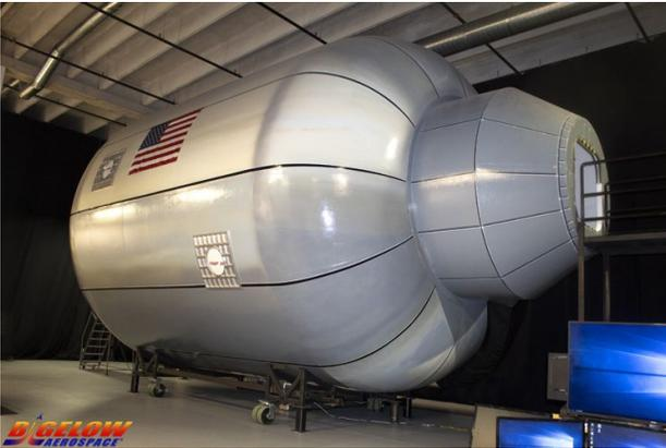
Fig. 8. Bigelow B330 inflatable habitat prototype [18].
