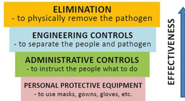
Figure 1. Hierarchical infection control pyramid, adopted from REHVA (2020), with four levels, for reducing the relative risk of airborne infection, where the top level is most effective and the bottom least effective.
