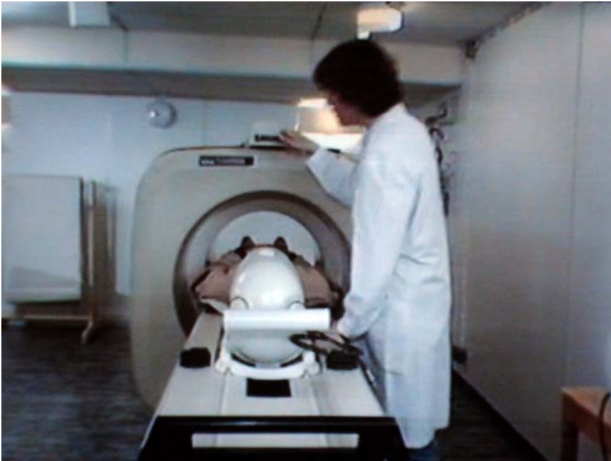
Figure 12. Staff guiding a patient into the MRI scanner at St. Görän's. The white helmet-like shape pointing towards the reader is a head coil. 37
