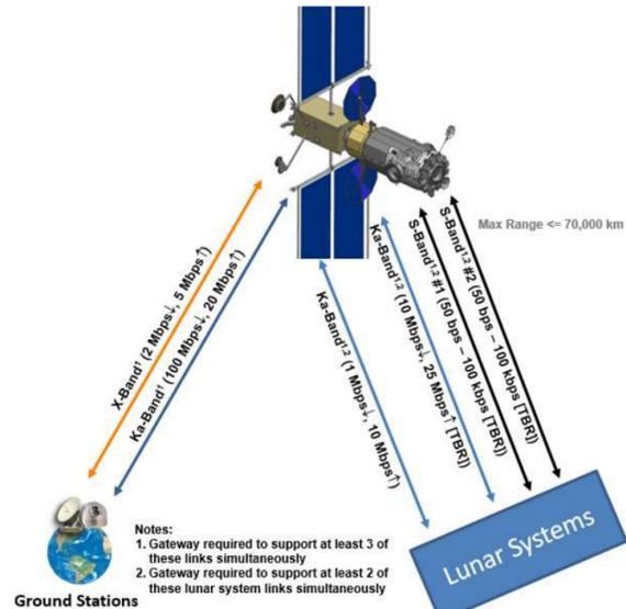
Fig. 6: 2024 Nominal Gateway Comm Architecture from NASA [19]
