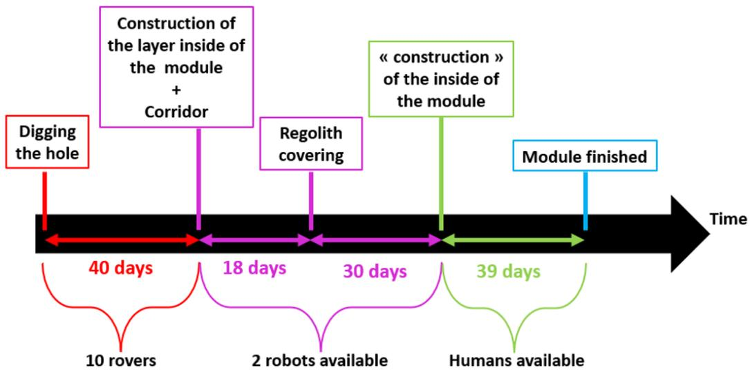
Fig. 8: Timeline of the construction of one module
