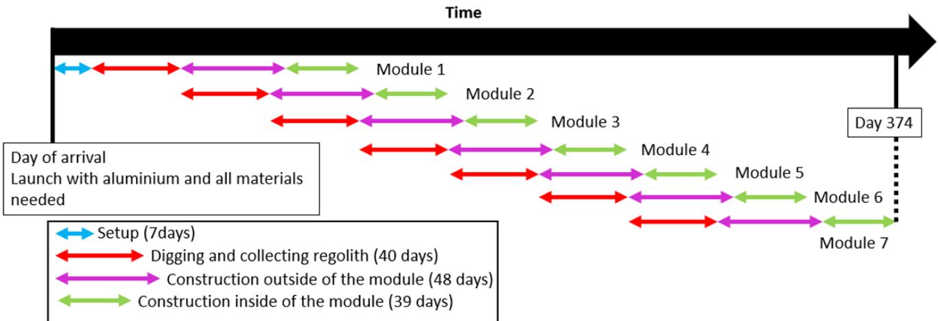
Fig. 9: Timeline of the construction of the base
