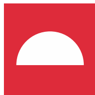
Other fire protection, possibly with additional sign, e.g., fire door, fire ventilation, smoke hatch or fire blanket
