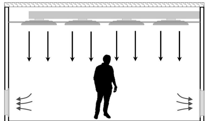
Fig. 5. Schematic of a unidirectional ventilation system.
