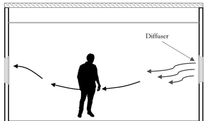
Fig. 7. Schematic of stratum ventilation.
