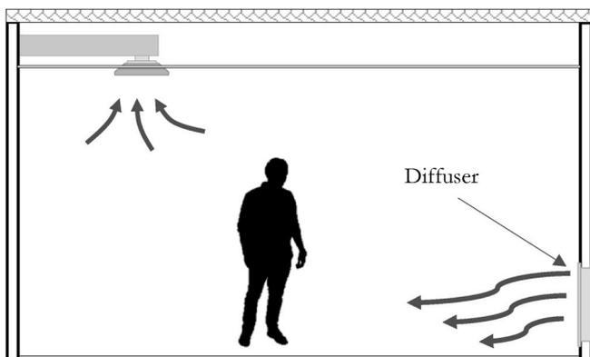
Fig. 6. Schematic of a displacement ventilation system.
