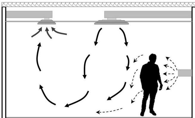
Fig. 8. Schematic of personalized ventilation.
