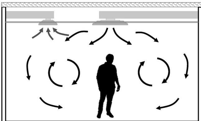
Fig. 4. Schematic of a mixing ventilation system.
