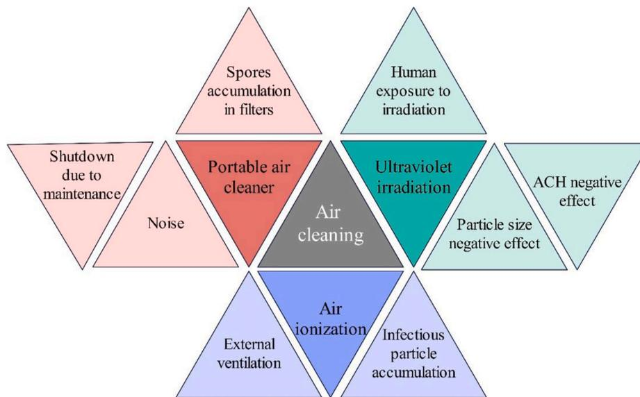
Fig. 10. Drawbacks and limitations of air cleaning approaches used in hospital wards.
