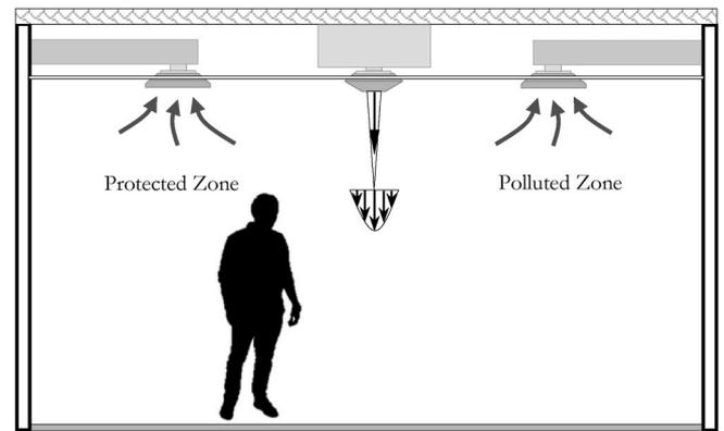
Fig. 9. Schematic of protected occupied zone ventilation.
