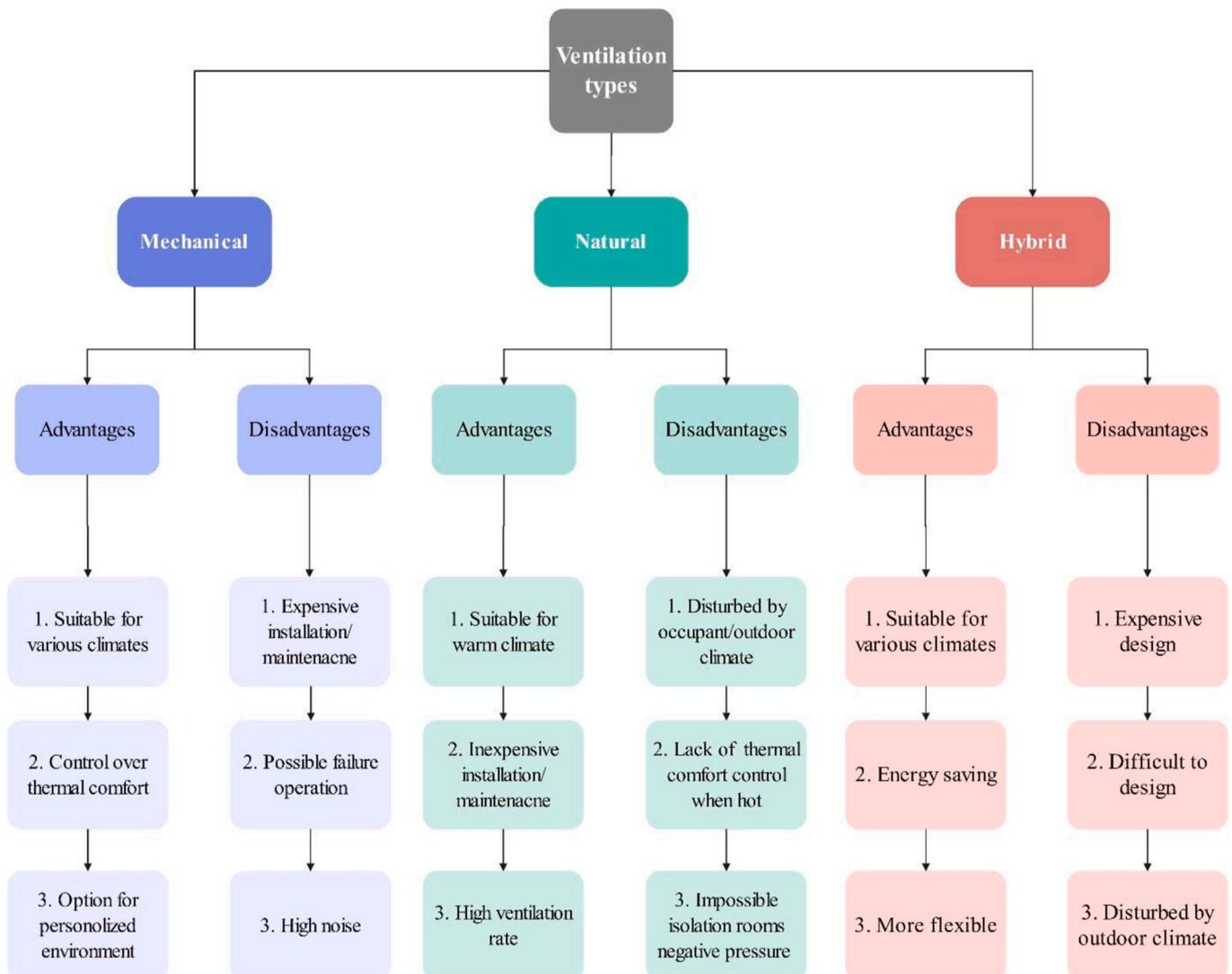
Fig. 2. Advantages and disadvantages of using natural, mechanical, and hybrid ventilation in hospital wards.
