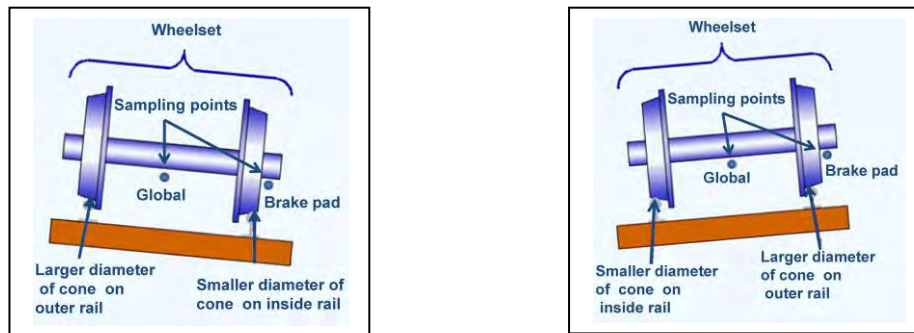
Fig. 19 Schematic showing position of sampling points, wheelset, and rail during curve negotiation: (a) right curve negotiation and (b) left curve negotiation
