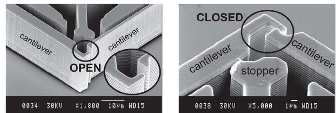
Fig. 8. Closeup view SEM pictures of the hook mechanism: (a) unlocked state (open switch), (b) locked state (closed switch).
