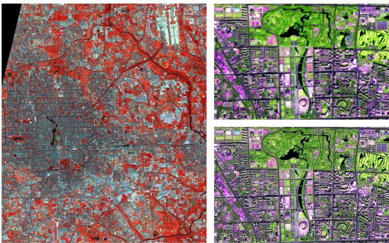
Figure 1. FCC Sentinel-2A image Beijing (left) and sub-scene before (upper right) and after pan-sharpening using band 8 (lower right).
