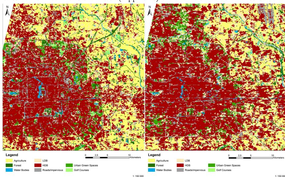
Figure 3. Classification result of Landsat TM data from 2005 (left) and Sentinel-2A MSI data from 2015 (right).
