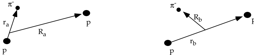
Figure 5.3. The Jacobian coordinate systems used. The origin of \mathbf{R}_i is at the center of mass of the two particles connected by \mathbf{r}_i .
