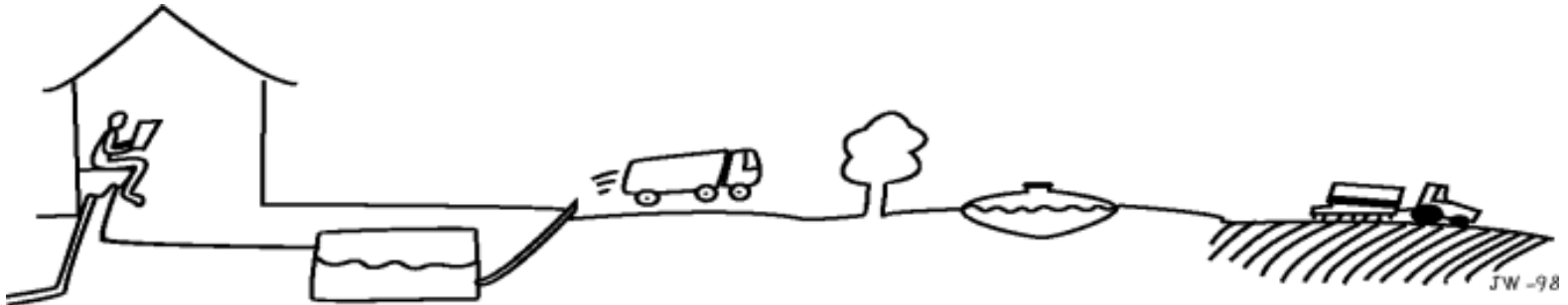
Example of system with Urine Diversion Dry Toilet (UDDT) and greywater management
