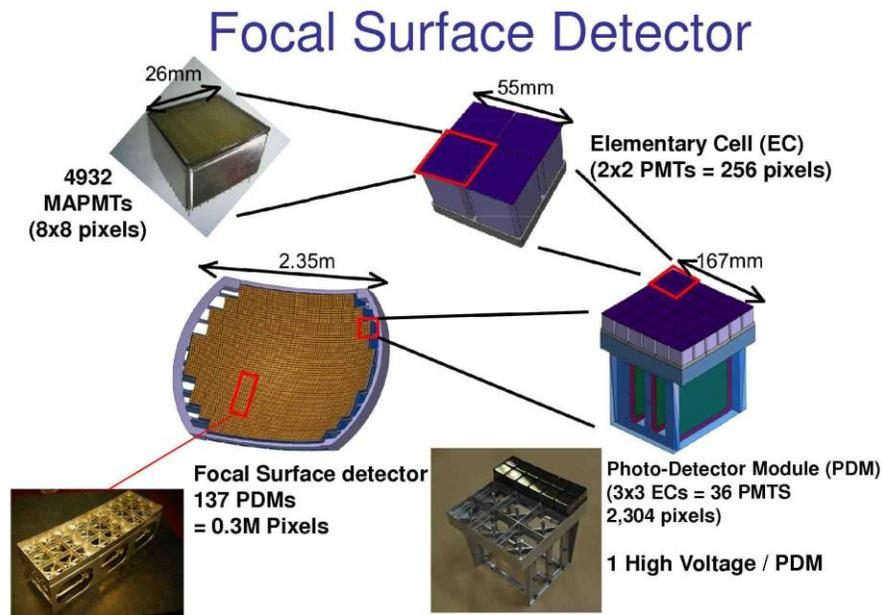
Figure 5 The breakdown of the JEM-EUSO focal surface into PDM, EC, and MAPMTs
