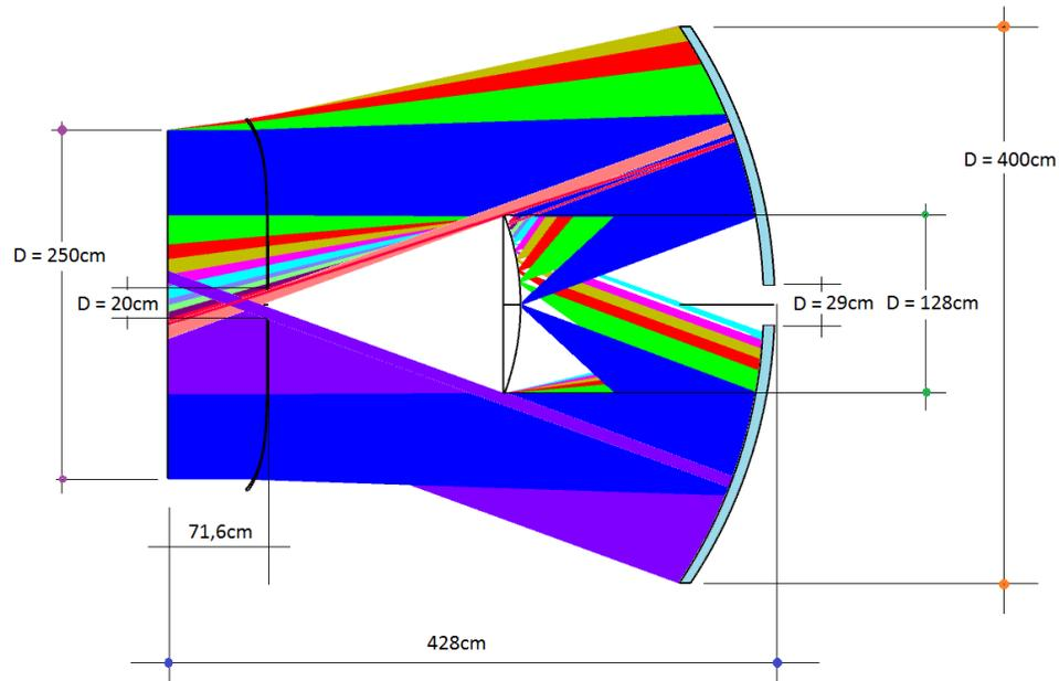
Figure 9 Schematic of the Schmidt telescope design of K-EUSO.
