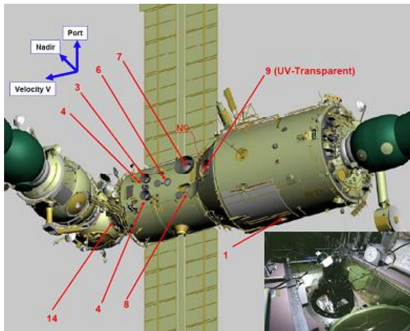
*Figure 6 Window number 9 is the UV-transparent window on the Zvezda module of the ISS. The inset shows the Relax experiment, previously mounted at the same window.*
