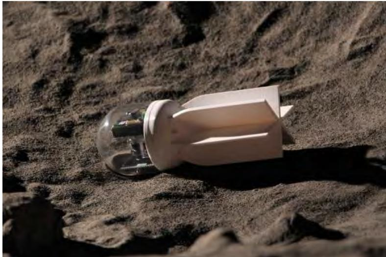
Figure 6.1: Deployed projectile mock-up microscope.
