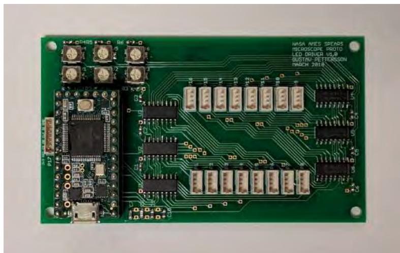
Figure 3.3: Control electronics for the microscope.
