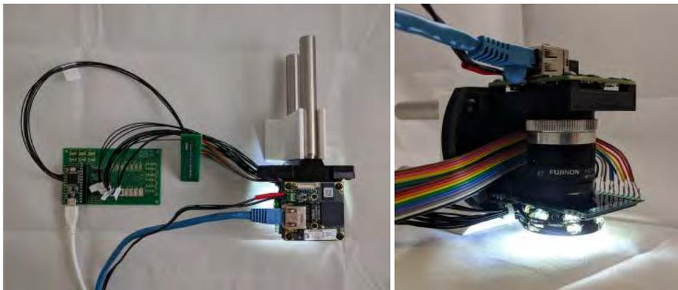
Figure 6.2: Assembled and connected optics.
