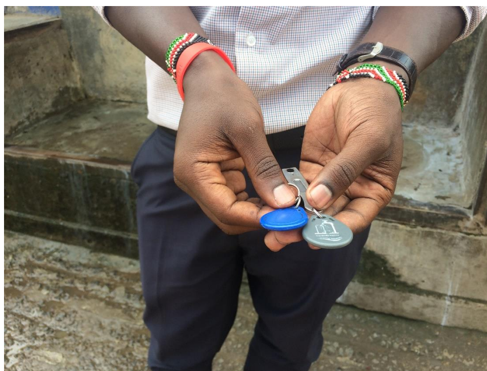
Figure 5. The electronic tokens or “shoptags” in Nairobi where water credit is stored. Photo: David Nilsson
